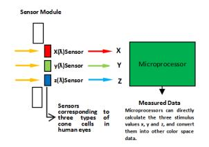
Figure E1 The principle of photoelectric integration method
