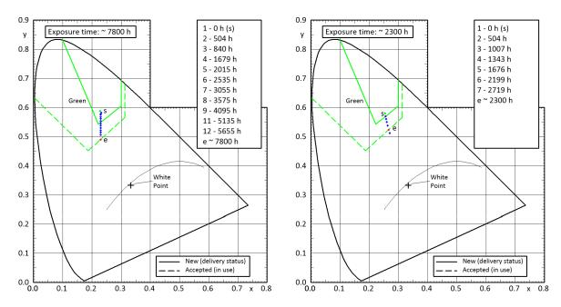
*Figure 13 CIE chromaticity diagram with measurements versus time (example from WSV, Germany)*
