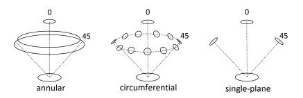
Figure 1 45° Illumination / 0° Measurement
