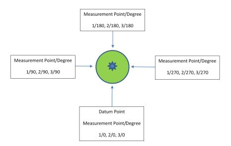
Figure 6 Top view of buoy with Datum Point and Measurement Points
