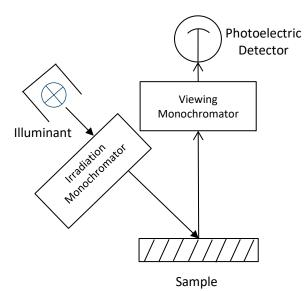
Figure D1 Component Parts of a two-monochromator system
