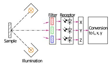
*Figure 3 Component Parts of a Colorimeter*
