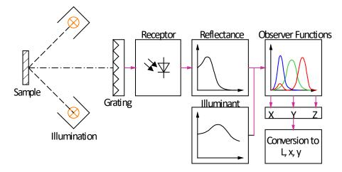
Figure 2 Component Parts of a Spectrophotometer
