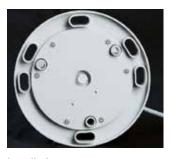
Installation The bottom plate of the LED110 supports installation on structure using 3 or 4 x M12 on a 200 mm diameter or 3 x M8 on a 150 mm diameter.
